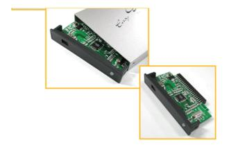
2. To connect between HDD and Easy Drive.
